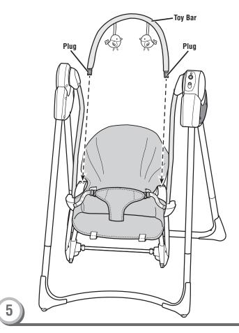
• Fit the plugs on each end of the toy bar into the sockets in each side rail.
